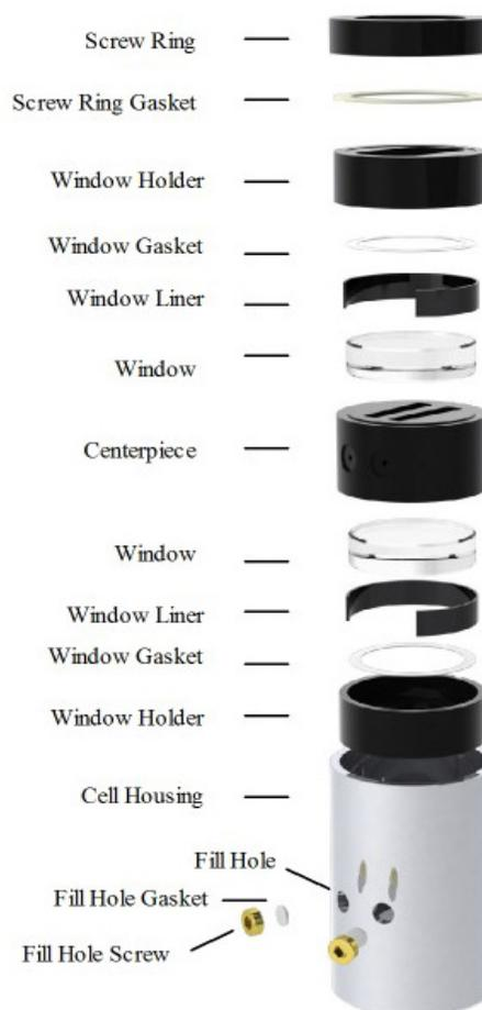
9. Screw the screw ring into the housing, making sure the word UP is facing you. (The word OUT is found on Beckman screw rings)
